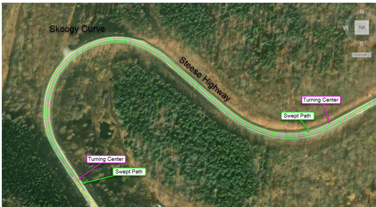
Figure 53: B-Train Swept Path Through Skoogy Curves Directions
