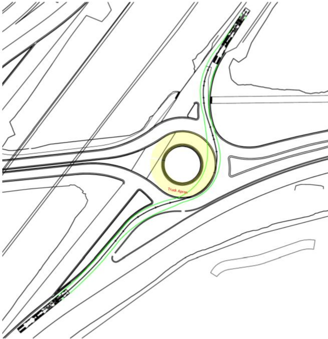
Figure 51: B-Train Turning Path Through Roundabout
