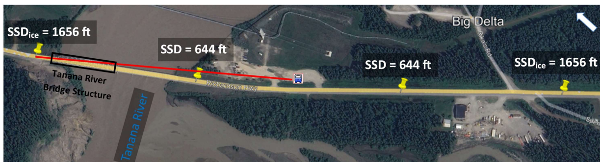
Figure 21: DGSD Richardson Highway Old Gas Station Stop at Bridge bus stop location
