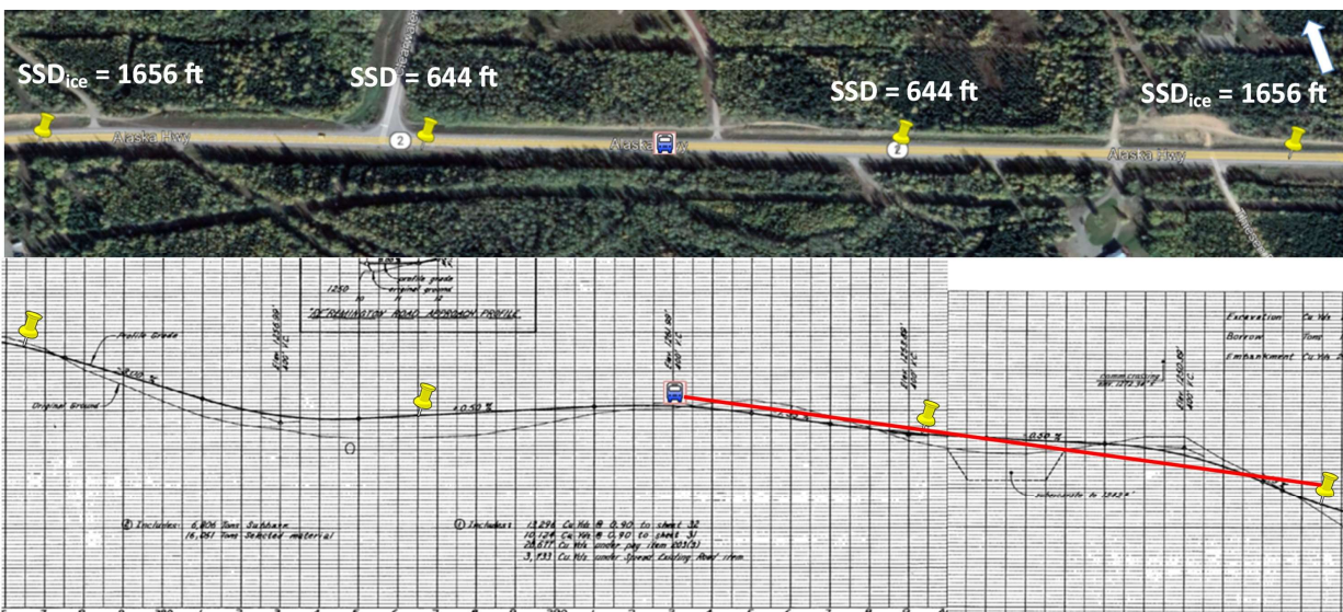
Figure 14: DGSD Alaska Highway at MP 1414.7 bus stop location
